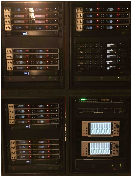
Firehouse Productions employed 62 channels of Sennheiser Digital 6000 wireless and 16 channels of Digital 9000 wireless to deliver pristine audio for Jesus Christ Superstar (Photo courtesy of Firehouse Productions)
